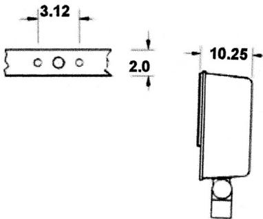
A 1000W floodlight for general purpose floodlighting applications with a wide-beam distribution. Available with Yoke mount or adjustable knuckle for 2" pipe mount.
